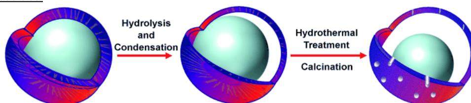
**A good egg:** A general and facile template strategy is presented for the fabrication of yolk-shell structures (see picture) with various types of movable cores, such as gold, SiO<sub>2</sub>, and magnetic Fe<sub>3</sub>O<sub>4</sub>. The vesicle template, formed of a fluorocarbon surfactant, is built up around the core.
