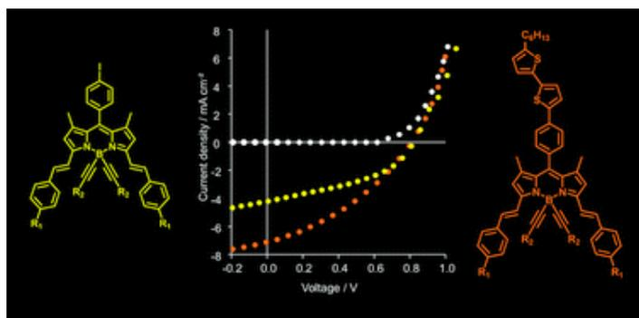
Fixation of a 5-hexyl-2,2-bithienyl unit on a conjugated BODIPY donor increases the conversion efficiency of the resulting molecular bulk heterojunction solar cells from 1.30 to 2.20%.
