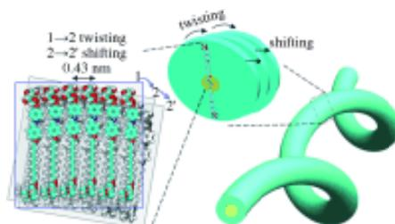
**Let's twist again!** A chiral rod-coil organometallic material, FC11, has been synthesized and shows liquid-crystalline behavior. By taking advantage of the self-assembly of the chiral Schiff based rod-coil molecule that is end-capped with ferrocene, the self-assembled superstructure can serve as a template to form iron-rich spiral superstructures (see graphic).
