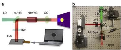
Customizing the output beam shape from a laser invariably involves specialized optical elements in
