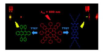
The phosphorescent metalloporphyrin sensitizer PtTPTNP (TPTNP = tetraphenyltetranaphtho[2,3]porphyrin) has been successfully coupled with perylenediimide (PDI) or rubrene utilized as triplet acceptors/annihilators to upconvert 690 nm incident photons into yellow fluorescence through sensitized triplet—triplet annihilation at overall efficiencies in the 6–7% range while exhibiting exceptional photostability.
