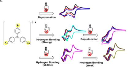
By increasing the number of amino substituents on triarylamine, the extent of hydrogen bonding between the oxidized form of triarylamine and imidazole could be electrochemically controlled.
