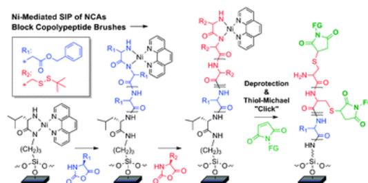
Homo-, block, and clickable copolypeptide brushes were synthesized using nickel-mediated surface-initiated polymerization of  $\alpha$ -amino *N*-carboxyanhydrides from low surface area substrates.
