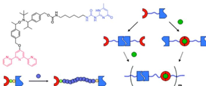
The synthesis of a new difunctional nitroxide initiator combining two orthogonal supramolecular entities is reported; controlled radical polymerization of styrene using this initiator is demonstrated to generate well-defined heterotelechelic polymers in a one-step procedure.
