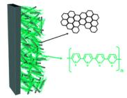
This communication reports on the development of high performance supercapacitor electrodes synthesized using a graphene/poly(pyrrole) composite layer.
