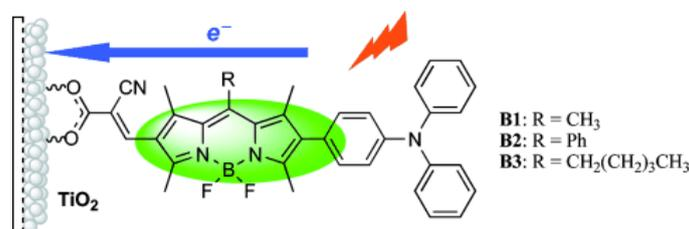
**Three novel 2,6-modified Bodipy sensitizers** were synthesized and evaluated for their use in dye-sensitized solar cells (DSSCs). Among them, dye **B3**, which carries a *n*-pentyl group at position 8, exhibits the best solar energy conversion efficiency (1.83 %). The results of this study provide a new strategy for the design of Bodipy derivatives as sensitizers for DSSCs.
