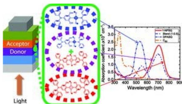
**Two squaraine (SQ) donor molecules with different absorption bands** are blended together for better coverage of the solar spectrum. The blend SQ device shows a significant improvement compared with single SQ donor devices. By applying a solvent annealing process and a compound buffer layer, a power-conversion efficiency of  $5.9 \pm 0.3\%$  is achieved under 1 sun illumination.
