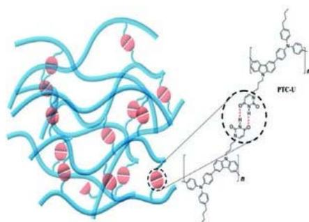
**A new DNA-mimetic  $\pi$ -conjugated polymer poly(triphenylamine-carbazole) (PTC-U)** has been prepared which exhibits high thermal stability, non-corrosion, excellent hole injection and electron-blocking abilities in the solid state owing to the uracil induced physical cross-linking. In addition, a trilayer device with PTC-U as a hole injection/transport layer is approximately 1.6 times higher than that of the commercial product PEDOT:PSS-based devices.
