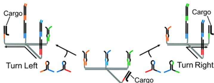
We have developed a programmable and autonomous molecular robot whose motion is fueled by DNA hybridization. Instructions determining the path to be followed are programmed into the fuel molecules, allowing precise control of cargo motion on a branched track.
