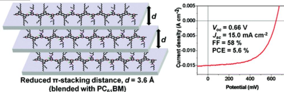
A series of semiconducting copolymers (PTAT-x) containing extended  $\pi$ -conjugated tetrathienoanthracene units have been synthesized. It was shown that the extended conjugation system enhanced the  $\pi$ - $\pi$  stacking in the polymer/PC61BM blend films and facilitated the charge transport in heterojunction solar cell devices. After structural fine-tuning, the polymer with bulky 2-butyloctyl side chains (PTAT-3) exhibited a PCE of 5.6% when it was blended with PC61BM.
