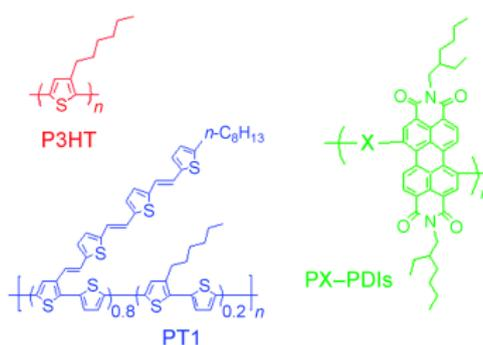
It's all about polymers: All-polymer solar cells (all-PSCs) based on six perylene diimide containing polymers (PX-PDIs) as acceptor materials and two polythiophene derivatives (P3HT and PT1) as donor materials were investigated systematically (see picture). The highest power-conversion efficiency (PCE) of all-PSCs was 2.23%, one of the highest PCEs of polymer/polymer blend photovoltaic devices reported to date.
