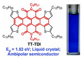
The first tetracene diimide derivative fused with four thiophene rings, TT-TDI, was synthesized by an FeCl<sub>3</sub> mediated oxidative cyclodehydrogenation reaction. TT-TDI exhibited a low band gap of 1.52 eV and amphoteric redox behavior. TT-TDI also showed a liquid crystalline property and ambipolar charge transport in thin film field-effect transistors.
