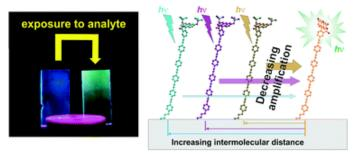
A simple method for tuning the performance characteristics of fluorescent ratiometric sensors based on surface-immobilized monolayers of  $\pi$ -conjugated molecules enabled gradual adjustment of the sensitivity and the analyte detection range of the sensor. This approach has been applied to fine-tune the sensing performance of a prototype ratiometric chemosensor for fluoride ions.
