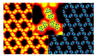
In this study, through the choice of the well-known G-K biological coordination system, bioligand-alkali metal coordination has for the first time been brought onto an inert Au(111) surface. Using the interplay between high-resolution scanning tunneling microscopy and density functional
