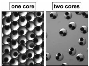
Monodisperse magnetic particles are templated from double emulsions formed using sequential flow-focus drop formation. The microfluidic drop formation allows the particles to be formed with high monodispersity and with consistently anisotropic internal structure. This structural anisotropy gives rise to magnetic anisotropy, allowing the particles to be rotated by a magnetic field.
