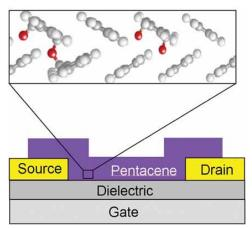
Electrical measurements of a pentacene (Pn) thin-film transistor reveal that oxygen exposure under certain bias voltages results in the formation of Pn gap states, whose influence on transistor properties is relevant to the development of organic electronics. A model explaining the origin of
