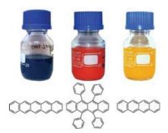
**Organic nanoparticle dispersions are prepared** via a versatile technique. Particles are formed by evaporation of aromatic hydrocarbons (like pentacene, rubrene, and tetracene) in an inert atmosphere and condensation of the vapor in a liquid medium. This allows the preparation of stable and concentrated dispersions of organic nanoparticles, showing interesting optical properties and potential applications in organic electronics and sensors.
