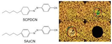
A new photoresponsive calamitic liquid crystal molecule possessing (1-cyclohexenyl)phenyldiazene as a close analogue of azobenzene was synthesized and a comparative study with the corresponding azobenzene analogue carried out.
