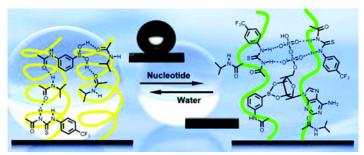
A smart copolymer film that is sensitive to nucleotide species in solution was developed. The film exhibits ann excellent reversible wettability response to nucleotide solutions, which is accompanied by a phase change and the corresponding swell and shrinkage of the copolymer.
