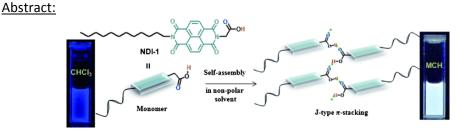
Almost pure white-light emission (fluorescence quantum yield=0.70) from a remarkably simple single-component, carboxylic acid appended naphthalenediimide (NDI) derivative has been reported. Aggregation-induced modulation of photophysical properties was attributed to hydrogen-bonding-mediated J-type  $\pi$  stacking among the NDI chromophores.
