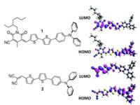
Improvements in the performance of small molecule-based organic solar cells have been reported through the use of a cyanopyridone acceptor group. This acceptor fragment enhances the absorbance of an oligothiophene-based dye and enables the addition of a solubilising alkyl chain that facilitates simple device fabrication from solution.
