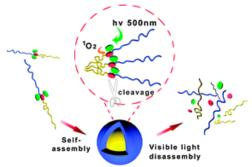
A class of dialkoxyanthracene-containing diblock copolymers is synthesized which possesses visible light-responsivity. These copolymers can self-assemble into a micellar structure in water. Green visible light (540 nm) is able to scissor these anthracene species and cleave the diblock copolymer into two fragments, inducing disassembly of the self-assembled micelles.
