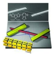
Ultrahigh-mobility organic field-effect transistors (OFETs) based on a CDT-BTZ donor-acceptor copolymer are realized by reaching high molecular order and pronounced alignment in single fibers within a short OFET channel via solution processing. The macromolecules directionally self-assemble in a quasi crystal-like order in the fibers providing in this way an unhindered charge carrier pathway with mobilities as high as  $5.5 \text{ cm}^2 \text{ V}^{-1} \text{ s}^{-1}$ .
