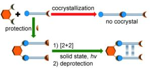
A supramolecular protecting group strategy has been applied to achieve solid-state photodimerizations of olefins lined with a combination of hydrogen-bond-donor and -acceptor groups. Esters were used as protecting groups to generate head-to-head photodimers that were readily converted into diacids. A protected olefin equipped with a stilbene unit exhibits enhanced reactivity that is ascribed to pedal motions in the solid state (orange hexagons: template: blur circles: recognition sites).
