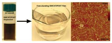
Single-walled carbon nanotube films are fabricated from a homogenous nanotube dispersion and a slow-evaporation technique. The transmittance and sheet resistance of the films are evaluated at room temperature. Using nanotube films as conductive substrates for electrochemical deposition illustrates that these nanotube films can act as alternatives to ITO for optoelectronic applications.
