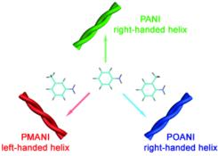
A game of Twister: The induced helicity of polyaniline and its supramolecular structures could be tuned by the methyl substitution of one of the monomers. By copolymerization of aniline with m-toluidine, the helicity of copolymer (PMANI) nanofibers was totally inverted compared to that of
