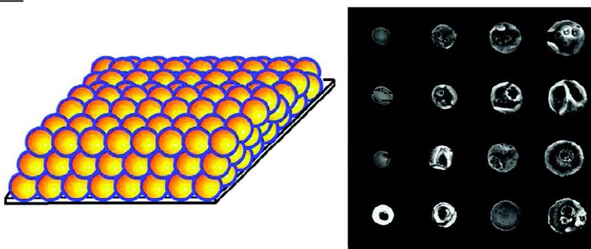
Thin films of gold on glass are prepared by solution deposition of functionalized gold nanoparticles followed by thermal treatment. The processed films adhere strongly to glass without any adhesion layers and can be micropatterned/ microetched without delamination from the substrate. The formation of self-assembled monolayers (SAMs) of oligo(ethylene glycol) alkane thiols (EG SAMs) renders the films resistant to cell adhesion and allows for cell patterning.
