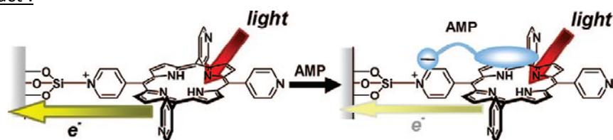
A 5,10,15,20-tetra(4-pyridyl)porphyrin (TPyP)-deposited ITO electrode as a sensor of nucleotides using photocurrent change was prepared. The TPyP-deposited ITO electrode could repeatedly detect nucleotides having concentrations of the  $\mu\text{M}$  order by a decrease in the photocurrent.
