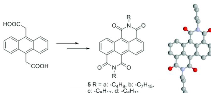
A successful synthesis of novel diimides, namely anthracene diimide containing six-membered imide rings, with potential application in organic electronics is reported. The single crystal of **5a** exhibits a close interplanar spacing of 3.45 Å between molecules in a stack.
