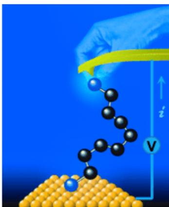
**Handling the (AFM) tip:** The duration of stable molecular junctions was prolonged using a tactile feedback method in which the operator can sense the force of the AFM tip on the sample surface (see picture). The movement of the tip is adjusted accordingly, maintaining a more consistent current ( $i$ ) and voltage ( $V$ ), instead of having the tip move at a constant preset speed, as in the conventional setup.
