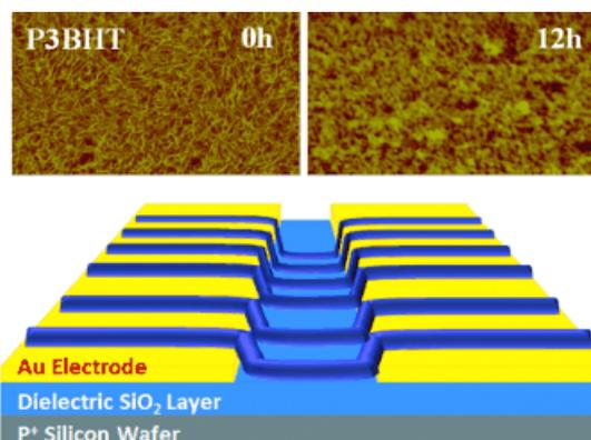
**Stripes on a plane:** A set of highly ordered microscopic stripes (purple; see scheme) were produced over a large area by using controlled evaporative self-assembly in a cylinder-on-Si geometry of conjugated homopolymers or all-conjugated diblock copolymer (P3BHT). The crystallinity of the as-prepared assemblies of P3BHT was greatly improved following chloroform vapor annealing, resulting in a fourfold increase in electrical conductivity.
