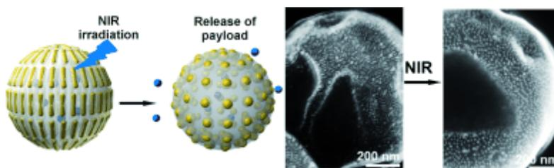
**The hydrodynamics of laminar flow** in a microfluidic device has been used to control the continuous self-assembly of gold nanoparticles (NPs) tethered with amphiphilic block copolymers. Spherical micelles, giant vesicles (500 nm–2.0 μm), or disk-like micelles could be formed by varying the flow rates of fluids. Such vesicles can release encapsulated hydrophilic species by using near-IR light (see picture).
