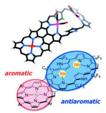
**Switch 'em up**: Two-electron oxidation and reduction switches the title complexes between aromatic and antiaromatic character (see picture). The switching is confirmed by <sup>1</sup>H NMR and UV/Vis/NIR absorption spectroscopy and by cyclic voltammetry. The structure of the porphyrin–[26]hexaphyrin hybrid tape was elucidated by X-ray diffraction analysis.
