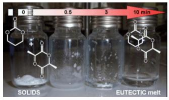
A 50:50 wt% mixture of L-lactide and trimethylene carbonate yields a eutectic at 21.3 °C.
