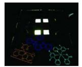
Highly efficient white organic light-emitting diodes (WOLEDs) with a simple, single-host-based structure are fabricated to realize the state-of-the-art performance of extremely low driving voltages, high efficiencies, and low efficiency roll-offs. This is the first single-host-based WOLED with both high efficiency and extremely low operating voltage at practical luminescence, demonstrating the great potential of these WOLEDs for portable display and lighting applications.
