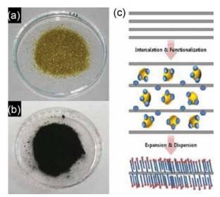
Easily soluble expanded graphite (see figure) is synthesized in a one-step exfoliation process that can be used for the lowcost mass production of graphene for various applications because of the simplicity and speed of the process. The graphene obtained is sufficiently expanded to be dispersed in aqueous solutions with an ordinary surfactant and in organic solvents.
