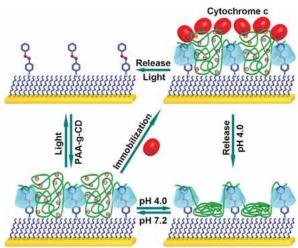
A light or pH dual-responsive reactivated biointerface is fabricated using of photocontrolled reversible inclusion and exclusion reactions between photoresponsive azobenzene-containing self-assembled monolayer and pH-responsive poly(acrylic acid) polymer grafted with cyclodextrins. The dual-controlled reactivated biointerface can be employed for reversible immobilization of redox protein-Cytochrome c, triggered by dual external stimuli-light and pH.
