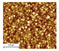
Under similar electrodeposition conditions the unique surface properties of pyrolyzed photoresist films result in smaller gold nanoparticles with a higher density when compared to other common electrode materials. Reactive ion etching of such surfaces results in the formation of unique AuNP-capped pyramidal carbon structures (see image).
