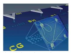
Carbon nanotubes are fabricated using chemical vapor deposition at predetermined locations by patterning catalyst directly on a substrate with nanometer-scale precision using dip-pen nanolithography with multipen cantilevers (see image). The development of new molecular inks for the deposition of the precursor catalyst results in a high yield of isolated carbon nanotubes, ideal for subsequent device fabrication.
