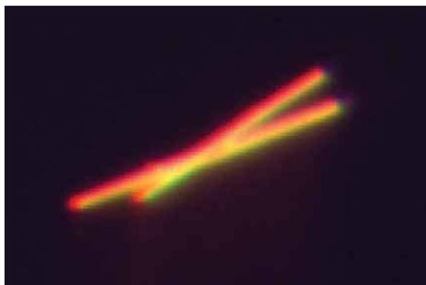
The open ends of oxide nanotubes (NTs) can be sealed with silica at room temperature and pressure after incorporation of desired materials into the NTs, the payload volume of which is adjustable (see picture for the case of fluorophores). This process originates from a synergetic reaction of capillary-condensed water and silicon reactants, which rapidly produces silica at the ends of the NTs.
