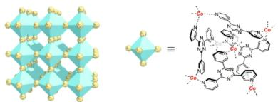
Reactive acrylate esters were encapsulated in the cavity of networked molecular capsules in a single-crystal-to-single-crystal fashion. Owing to the encapsulation effect, acrylates inside the capsules do
