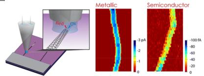
We introduce a multiprobe platform for the investigation of single-walled carbon nanotubes (SWNTs) that allows the electrochemical response of an individual SWNT to be mapped at high spatial resolution and correlated directly with the intrinsic electronic and structural properties. With this approach, we develop a detailed picture of the factors controlling electrochemistry at SWNTs and propose a definitive model that has major implications for future architectures of SWNT electrode devices.
