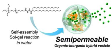
Semipermeable organic-inorganic hybrid vesicles coated with a siloxane surface were spontaneously formed by simple dispersion of an organoalkoxysilane lipid in water. The hybrid vesicles allow the permeation of hydrophilic small molecules across the membrane without an introduction of a poreforming protein.
