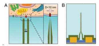
The miniaturization of bioelectronic intracellular probes with a wide dynamic frequency range can open up opportunities to study biological structures inaccessible by existing methods in a minimally invasive manner. Here, we report the design, fabrication, and demonstration of intracellular bioelectronic devices with probe sizes less than 10 nm. The devices are based on a nanowire—
