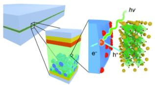
**Switching to solids:** Solid-state dye-sensitized solar cells are achieving efficiencies similar to those of their counterparts with liquid electrolytes. The new p-type semiconductor CsSnI3 was found to be an excellent replacement for the traditional  $I^-/I^{3-}$  redox system. The picture shows a cross section of a dye-sensitized solar cell based on CsSnI<sub>3</sub>.
