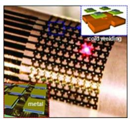
Strategies are presented to achieve ultrathin light-emitting diodes using the technique of epitaxial liftoff in ways that protect the materials from the etchants used for release and tether the devices to the underlying wafer for subsequent transfer printing onto substrates of interest. The results lead to an advanced interconnection scheme and vertical device layout that facilitate electrical contacts and system integration on flexible substrates.
