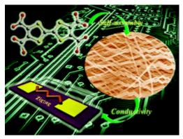
Quasi-one-dimensional electroactive materials with zigzag shape are fabricated by supramolecular self-assembly of a tetrathiafulvalene (TTF) derivative and metal ions under mild conditions. This is the first time that self-assembled organic conductors with zigzag shape are reported.
