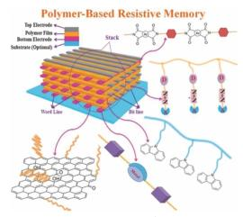
In this review we introduce the general characteristics of the device structures and fabrication, memory effects, and switching mechanisms of polymer-based resistive memory devices. Subsequently, the research progress concerning the use of single polymers or polymer composites as active materials for resistive memory devices are summarized. Finally, current challenges and future research directions in this field are discussed.
