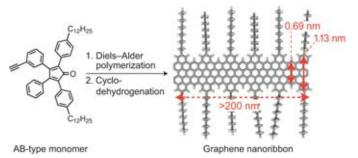
Liquid-phase-processable graphene nanoribbons (GNRs) over 200 nm long and with well-defined structures have now been synthesized by a bottom-up method, and are found to have a large optical bandgap of 1.88 eV. Scanning probe microscopy revealed highly ordered self-assembled monolayers of the GNRs, and the high intrinsic charge-carrier mobility of individual ribbons was characterized by terahertz spectroscopy.
